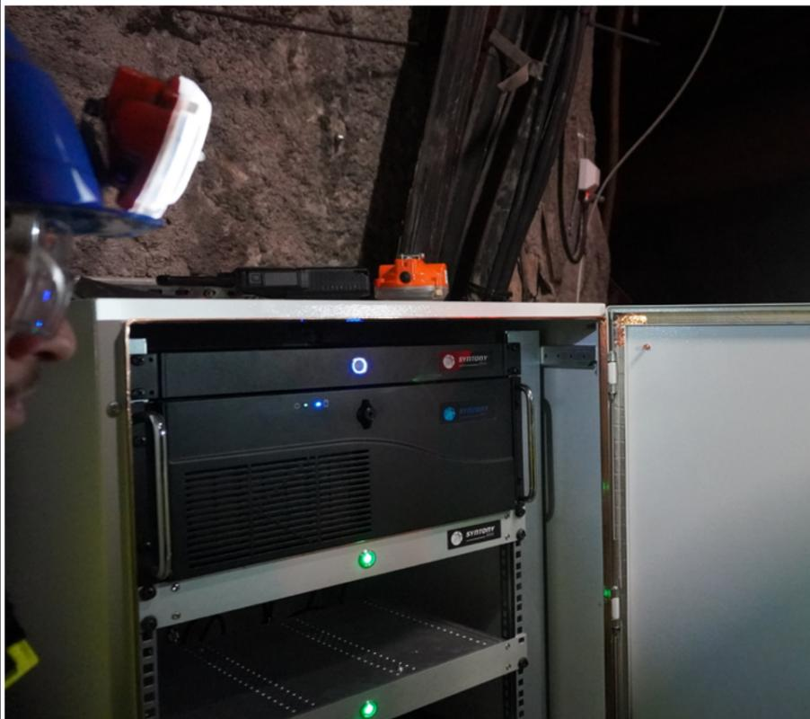
SubWAVE™ is a real-time GPS\* emulator providing signal in facilities out-of-range from natural GPS.
